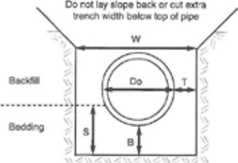
Do not lay slope back or cut extra trench width below top of pipe
