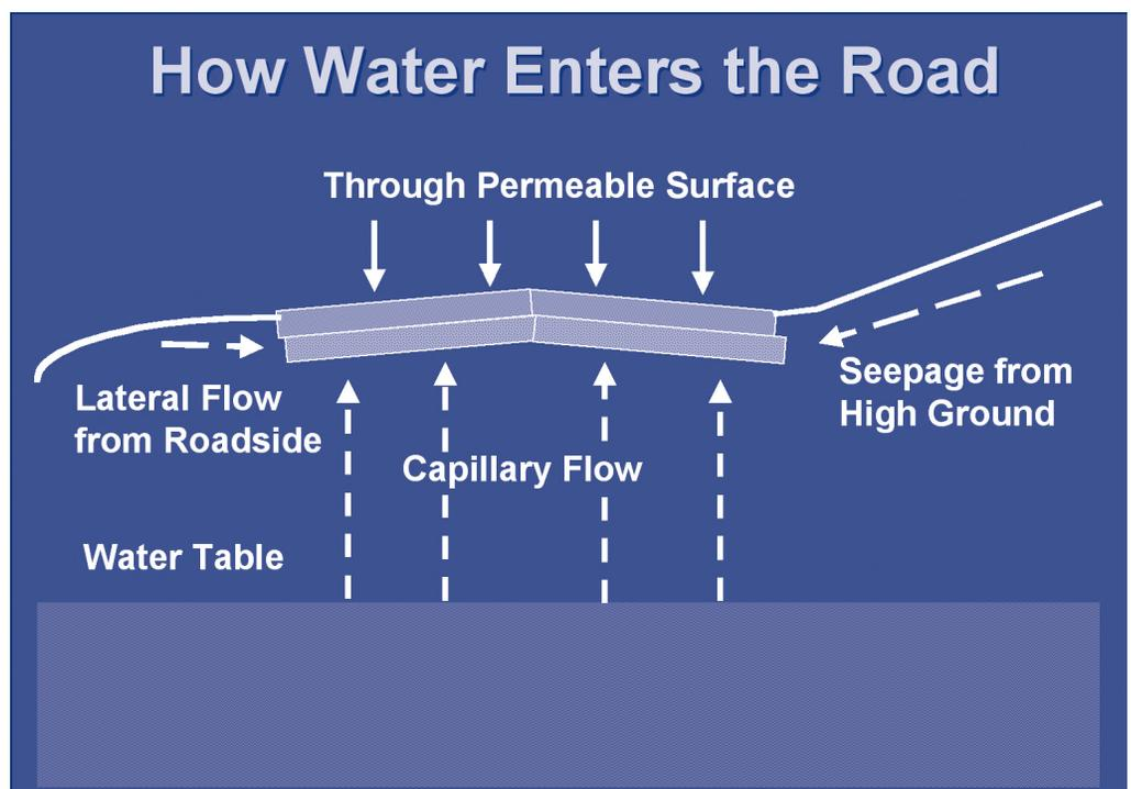
A surface drainage system has four components: road crown, shoulders, ditches, and culverts.
