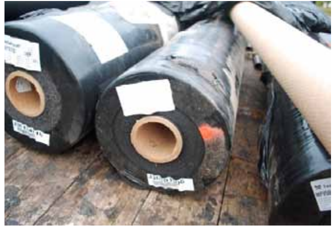
Geotextile rolls must be stored off the ground and adequately covered to protect them. Photo courtesy of ISMF LLC.
