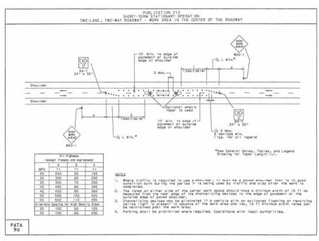
what advance warning and regulatory signs (per MUTCD) are necessary, the distance required for advance warning sign placement (A), the maximum distance between channelizing devices (D), the required taper length (L), whether a shadow vehicle or vehicles are required, and what distance (E) is desired between the shadow vehicle and the end of the taper.
