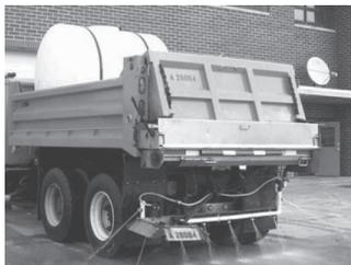
**Anti-icing material from straight-stream nozzle.**
