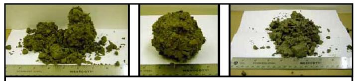
A hand-compacted ball can be used to estimate moisture. DSA that is too dry crumbles (left), DSA at optimum moisture retains a ball shape (middle), and DSA that is too wet will not compact (right).
