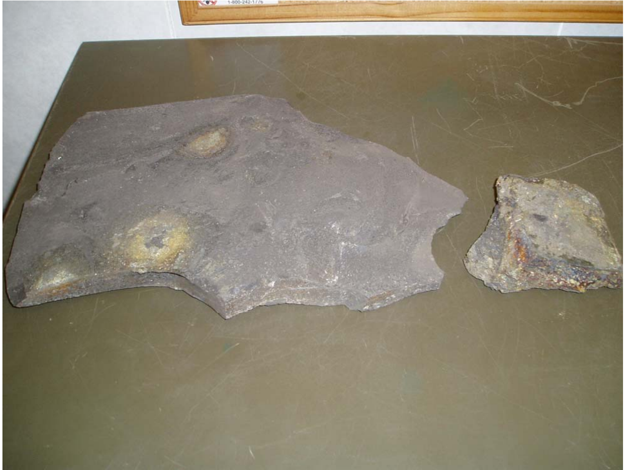
Figure 5.3. Pyritic black shale samples taken from beneath heaved floor slabs at the Evangelical Hospital in Lewisburg, Pennsylvania (S.E. Hoover, Pers. Comm., 2007).
