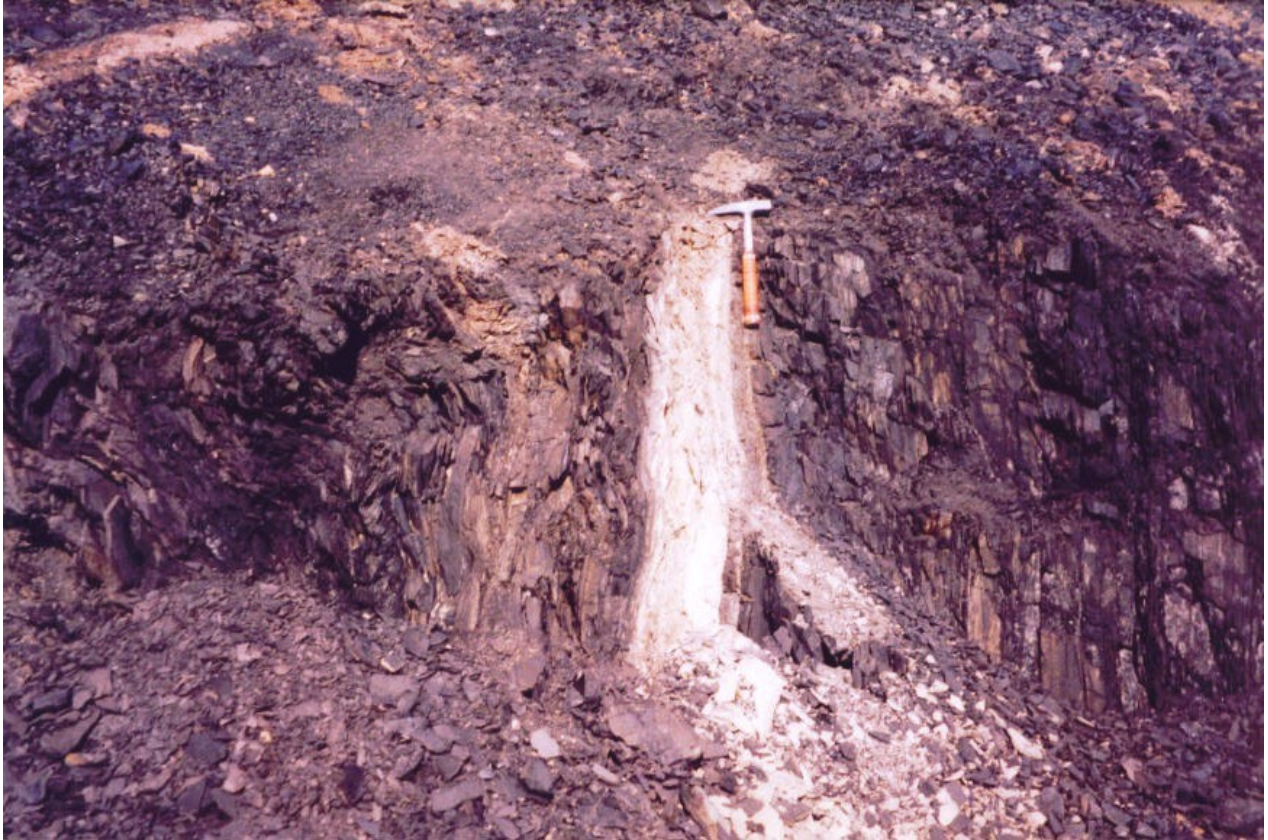
Figure 5.5. Photograph showing exposure of the near vertical black shale of the Marcellus Formation and one of the light colored Tioga ash beds exposed during construction along Route 522 west of Lewistown, Pennsylvania.
