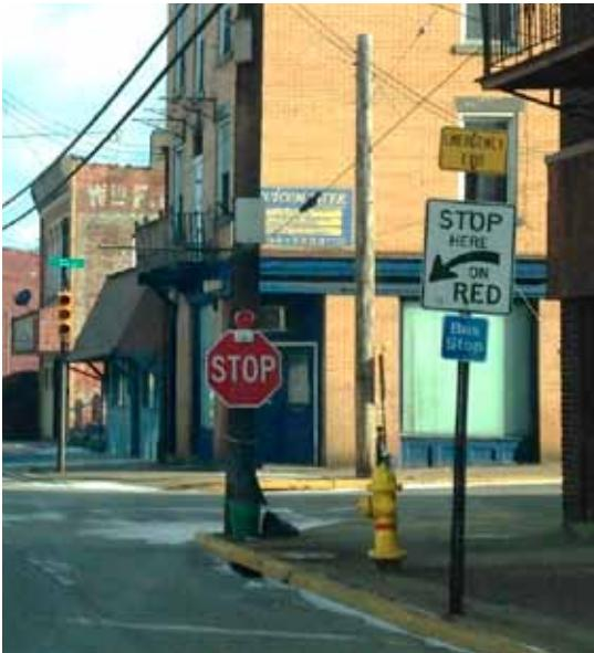
Cluttered streets can make sign placement challenging. Signs may be erected on existing poles as long as their placement meets all state and federal criteria, including mounting height, lateral offset, and longitudinal placement. The stop sign shown here does **not** meet the placement criteria.
