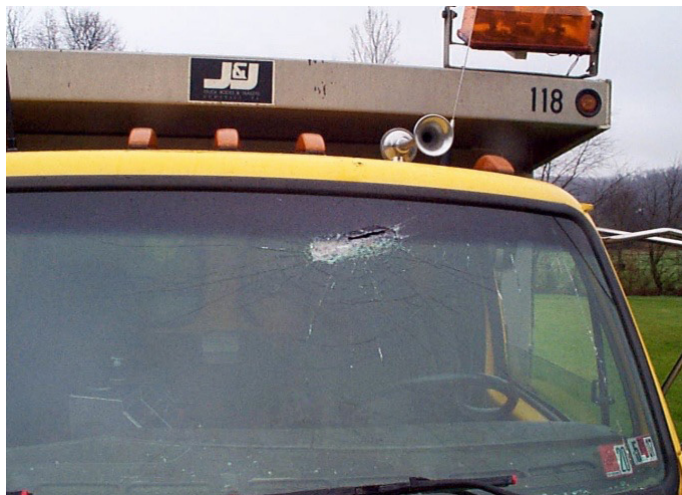
Check moving parts on a piece of equipment to ensure that all bolts/nuts are properly tightened. A loose blade from a mower will ruin the day of anyone or anything that gets in its way.
