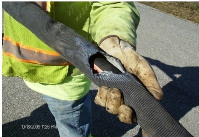
Replacing a damaged outer cover can be done at a fraction of the cost of replacing the entire hose.
