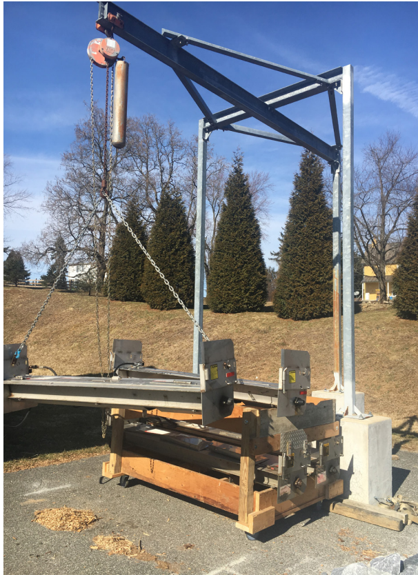
The East Brandywine Township road crew designed and built a portable storage rack for spreaders out of scrap lumber and inexpensive wheels. A hoist lifts the spreaders for mounting on trucks.
