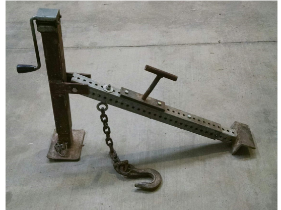
Using an old stop sign post, a car jack, and a chain with a hook, two employees at the City of Easton engineered a device that easily removes storm sewer inlet covers for inspection and cleaning. The tool is placed over the inlet grate with the angle iron against the curb. The hook is attached to the grate, and the handle is cranked to lift the cover.
