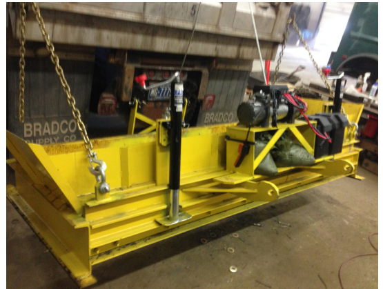
The City of Williamsport's public works department created the Polish paver, which attaches to a truck and more efficiently lays blacktop to repave roads and repair potholes.
