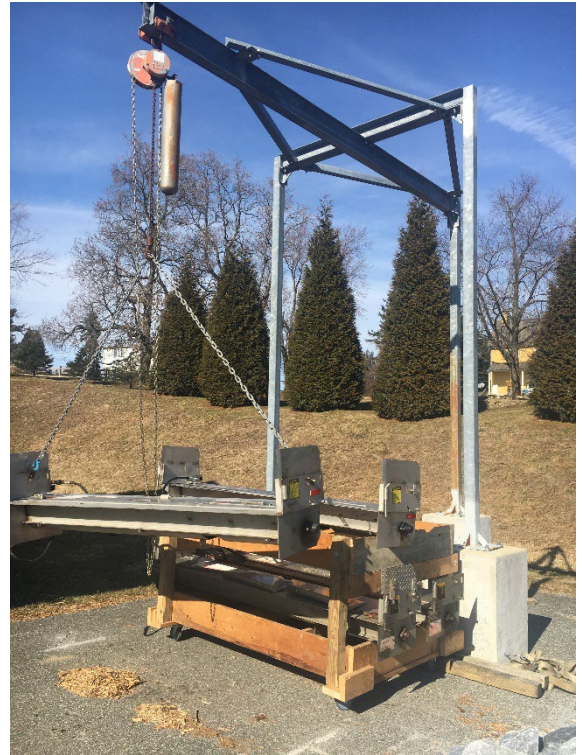
The East Brandywine Township road crew designed a portable storage rack for spreaders out of scrap lumber and inexpensive wheels. A hoist lifts the spreaders for mounting on trucks. (Credit: Matthew VanLew, East Brandywine Township, PA)
