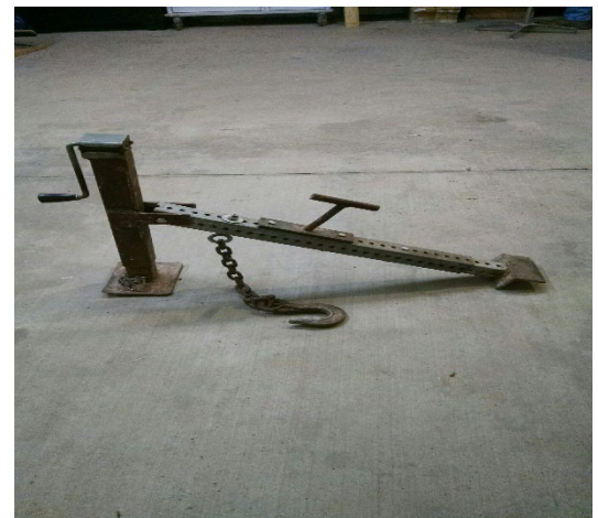
Using an old stop sign post, a car jack, and a chain with a hook, two employees at the City of Easton engineered a device that easily removes storm sewer inlet covers for inspection and cleaning. The tool is placed over the inlet grate with the angle iron against the curb. The hook is attached to the grate, and the handle is cranked to lift the cover. (Credit: Dwayne Woolverton & Bob Piperato, City of Easton, PA)
